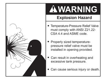
This water heater is provided with a properly rated/sized and certified combination Temperature-Pressure Relief Valve (T&P valve) by the manufacturer. The valve is certified by a nationally recognized testing laboratory that maintains periodic inspection of production of listed equipment of materials as meeting the requirements for Relief Valves for Hot Water Supply Systems, ANSI Z21.22 • CSA 4.4, and the code requirements of ASME.
